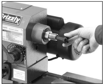
Figure 8. Installing the spur center.
